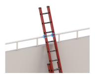
Figure 11 Correct - tying near the base
