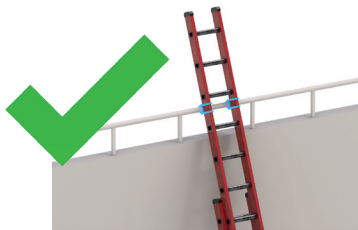
CORRECT - tied at top stiles
